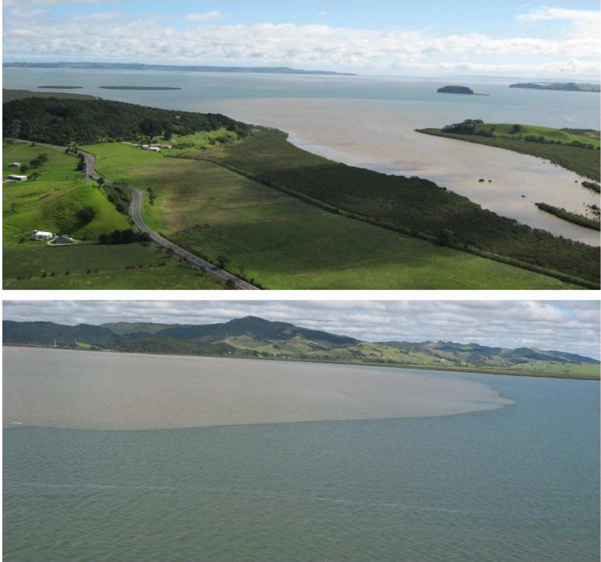
Figure 3-11: Plume of silt-laden flood water dispersing widely from the Hoteo River mouth on the ebb tide, 22nd March 2011, at 2:40 pm. Upper photo looking northwest towards the entrance to the Kaipara Harbour; Lower photo looking northeast across the southern Kaipara Harbour to the Hoteo River mouth. (Photos: Mark Pritchard, NIWA).
