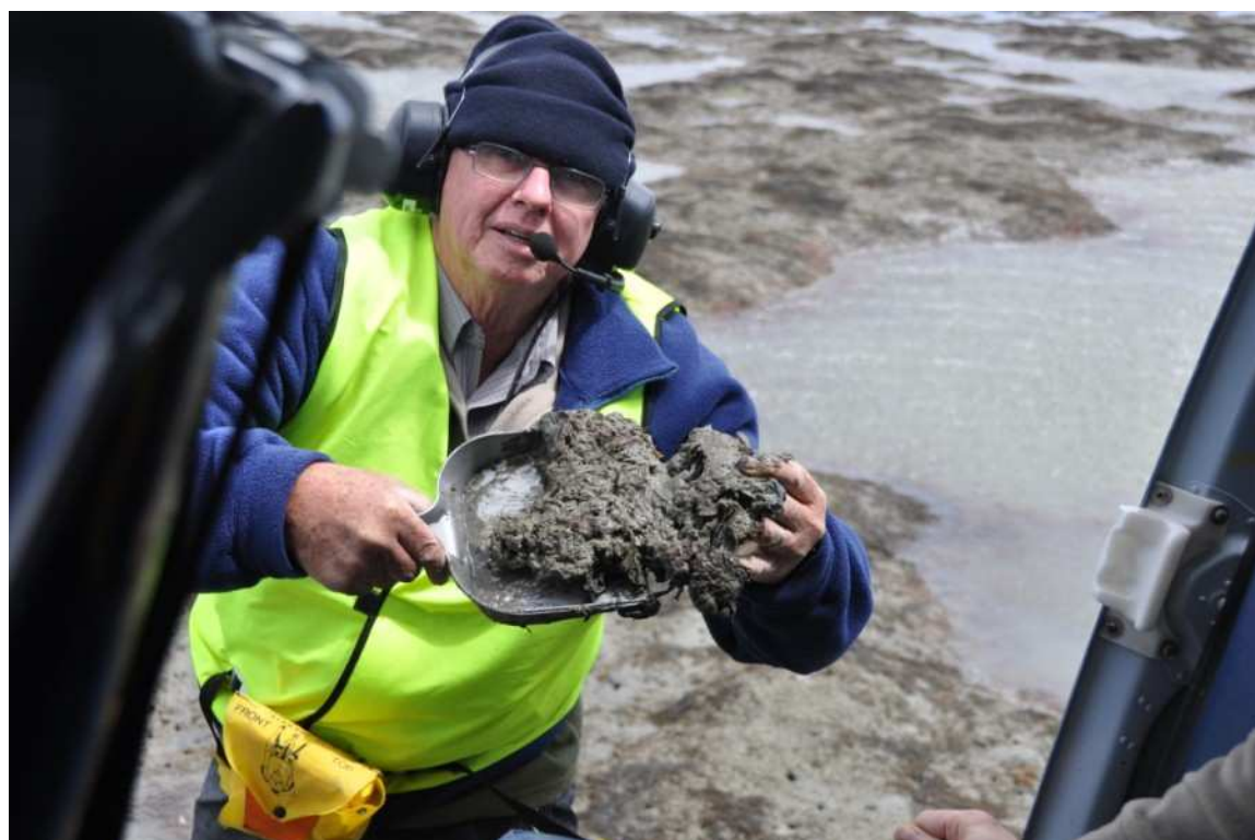
Figure 2-2: Sediment sampling. Plastic sampling scoop was 150 mm wide with a 20 mm high back. Multiple divots were placed in the plastic bag. The sample shown is an Asian mussel mat ( Musculista senhousia ). [Subject: Max Gibbs; Photo: Luca Chiaroni, NIWA].
