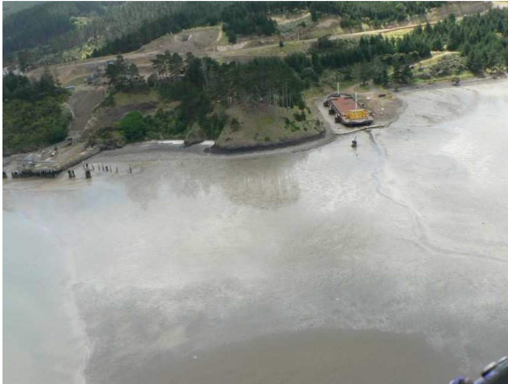
Figure A-18: Infrastructure along the shoreline of the northern Kaipara Harbour. Unsealed roads, quarries and the loading facilities for the barge represent potential sources of localised sediment erosion.
