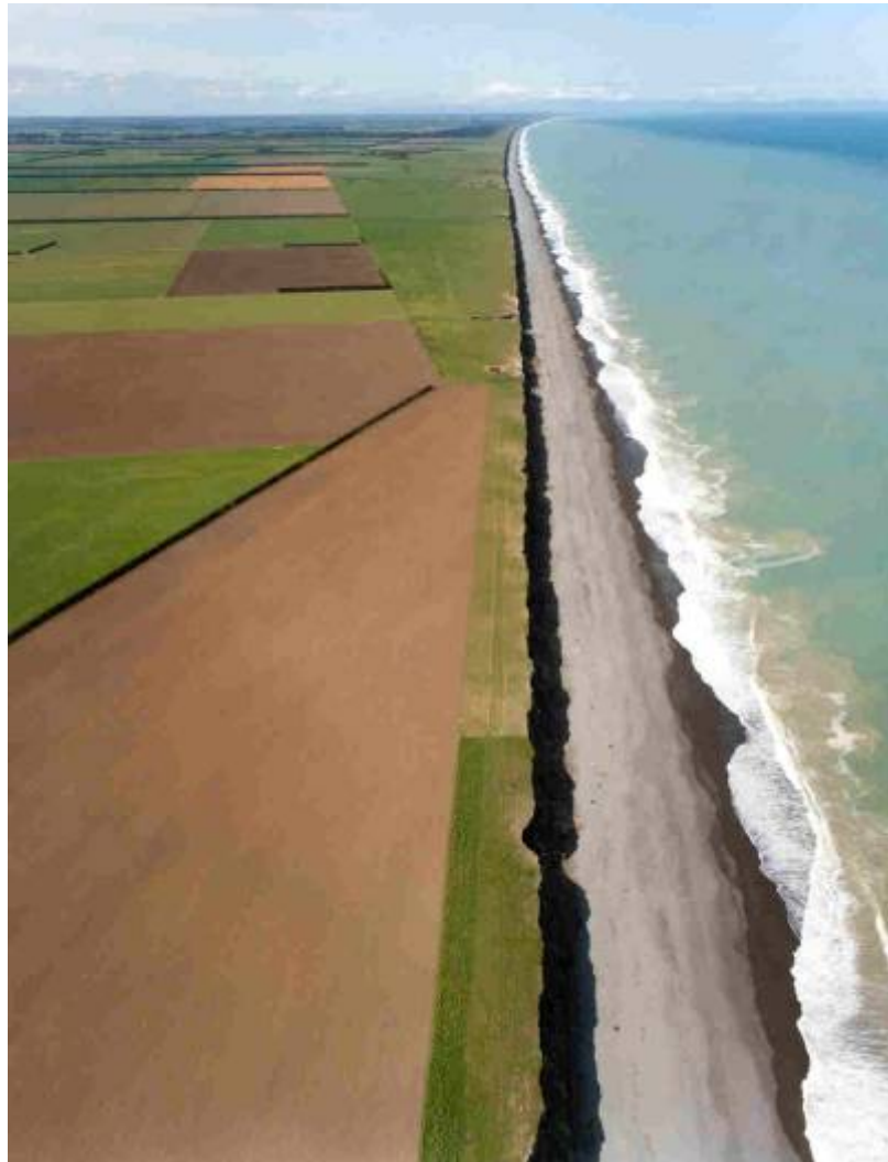
Figure 9: Near-shore suspended sediment fringe due to erosion of near-shore seabed and step (formed in the Pleistocene, 5.1–1.81 million years ago) outwash gravels along the South Canterbury coast. (Source: Environment Canterbury.)
