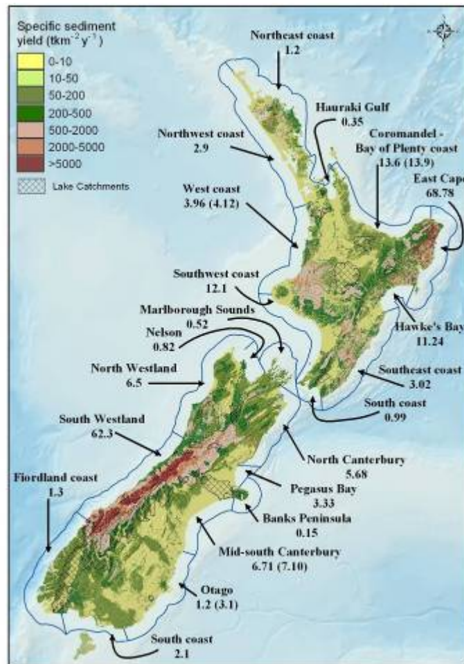
Figure 3: Annual present-day suspended sediment yields into different coastal areas of New Zealand. Numbers given are tonnes × 10 6 per year; bracketed figures are predicted yields if rivers had no dams on them. (Source: Murray Hicks, NIWA.)
